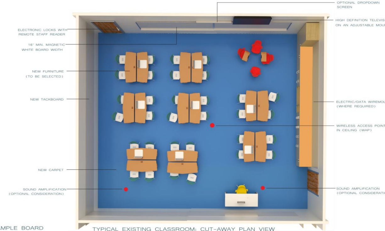
TYPICAL EXISTING CLASSROOM: CUT-AWAY PLAN VIEW
